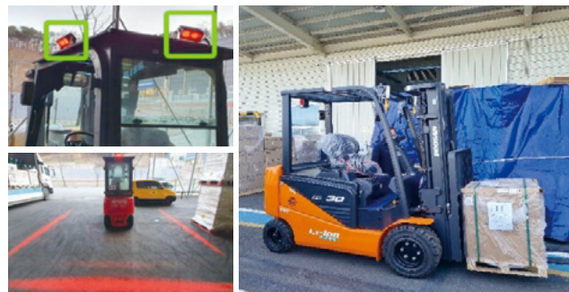
Lithium-powered forklift with safety devices installed
