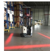
Forklift Operating Area Guide Line
