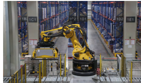
Layer picker in Yangsan Integrated Automation Center
