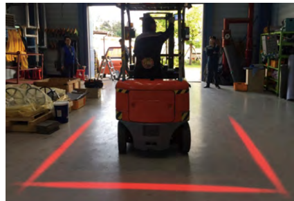
Forklift LED safety line
