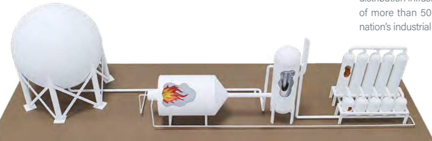
Pilot plant model for clean hydrogen production from pyrolysis-based ammonia
