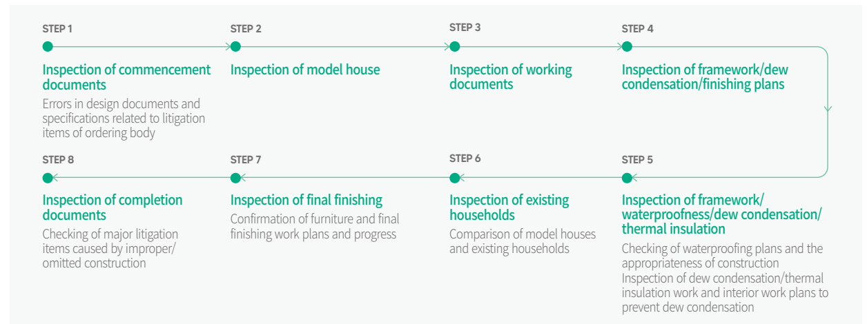
Quality inspection process of housing construction site
