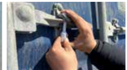
컨테이너 봉인(Seal) 개선(High Security Bolt type)
