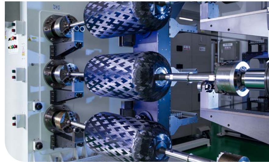
1 LOTTE Chemical, Dry filament winding of hydrogen tank
